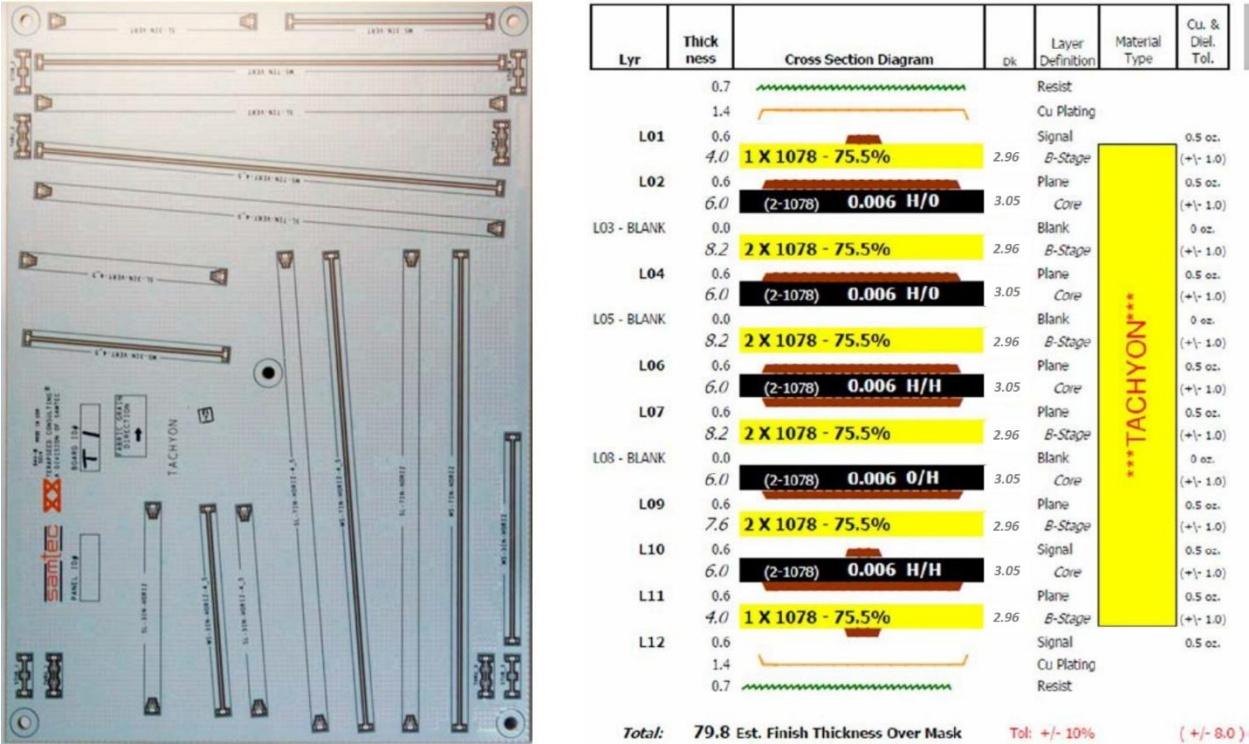
Figure 13 Test vehicle PCB and stackup reference DesignCon 2015 paper [5].
