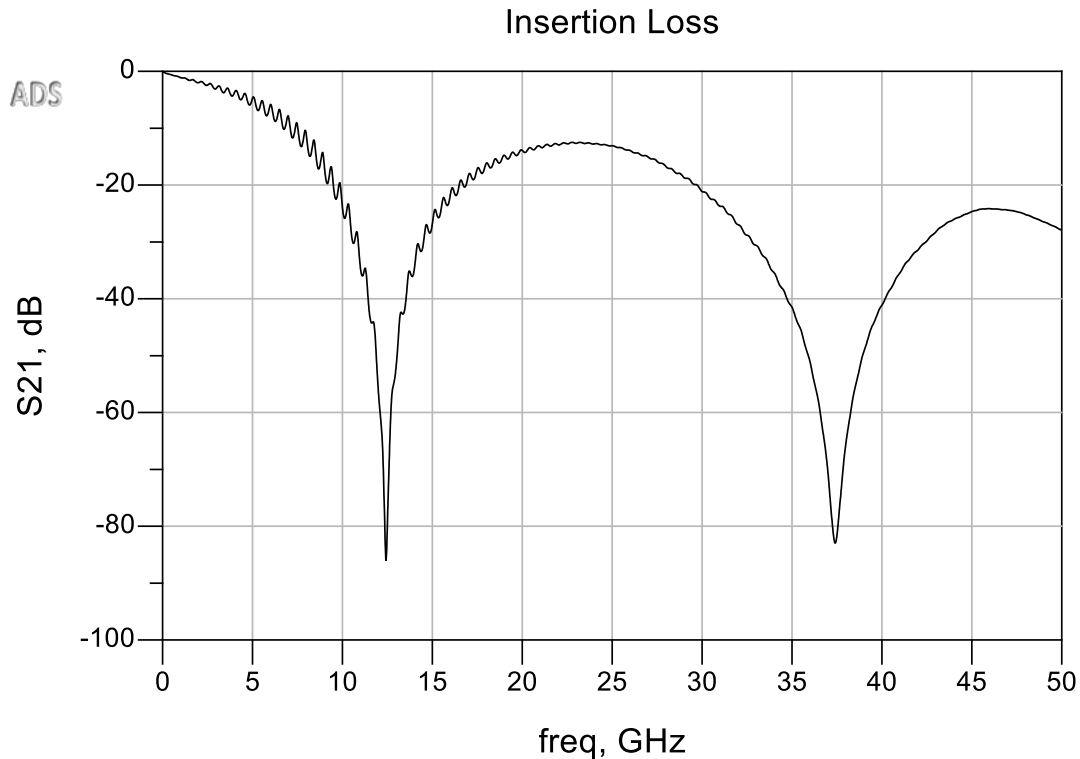
Figure 1 S21 Insertion loss plot showing resonant nulls due to quarter-wave stub resonances.
