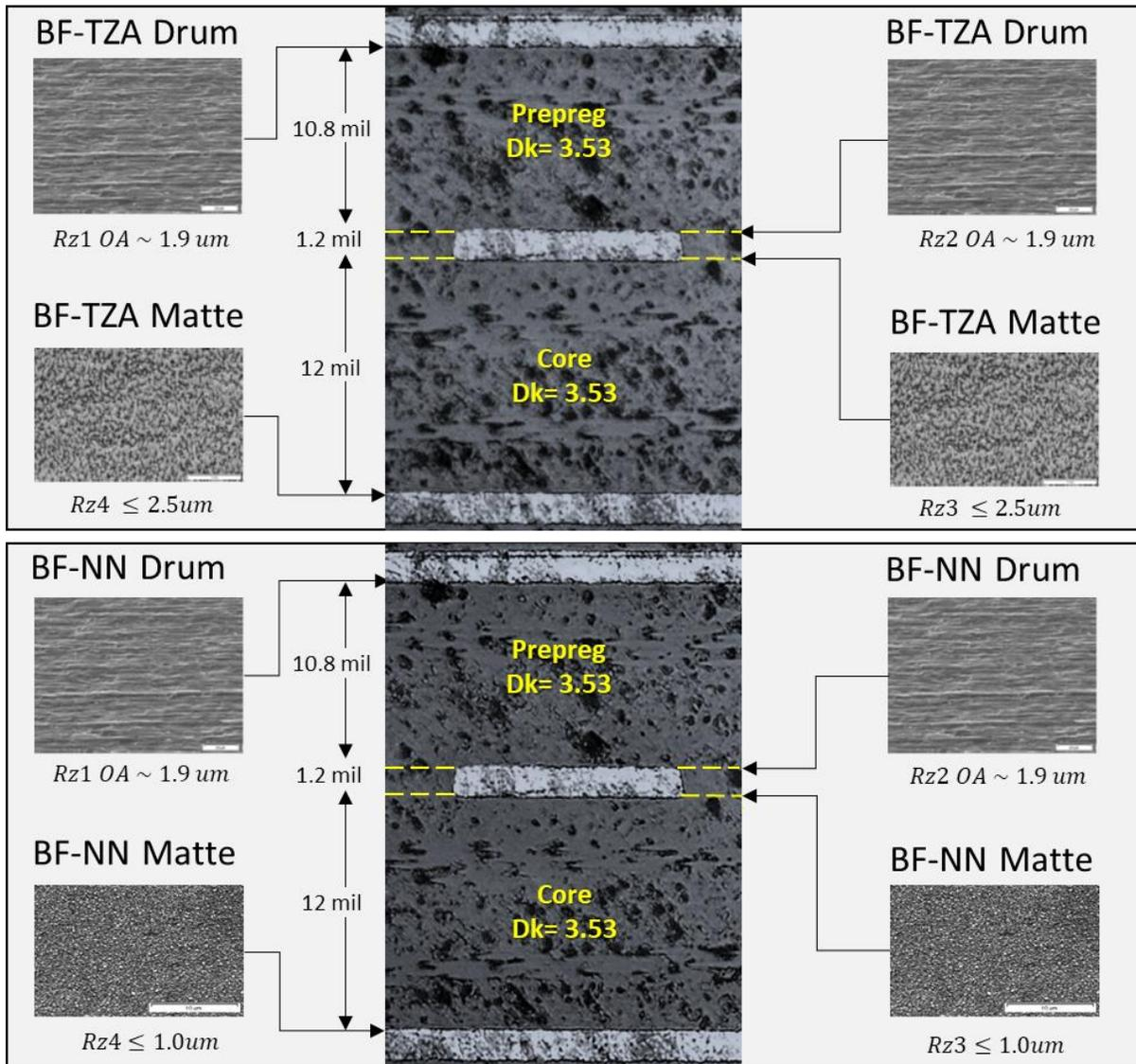
**Figure 14** Alternate foil options simulated for what-if loss comparison. Top is VLP2/VLP2 foil parameters for all copper layers and bottom is VLP1/VLP1 foil parameters for all copper layers. Note: Photos are for illustrative purposes only and are not actual cross-section from CMP PCB. Surface roughness pictures source: Circuit Foil [7]
