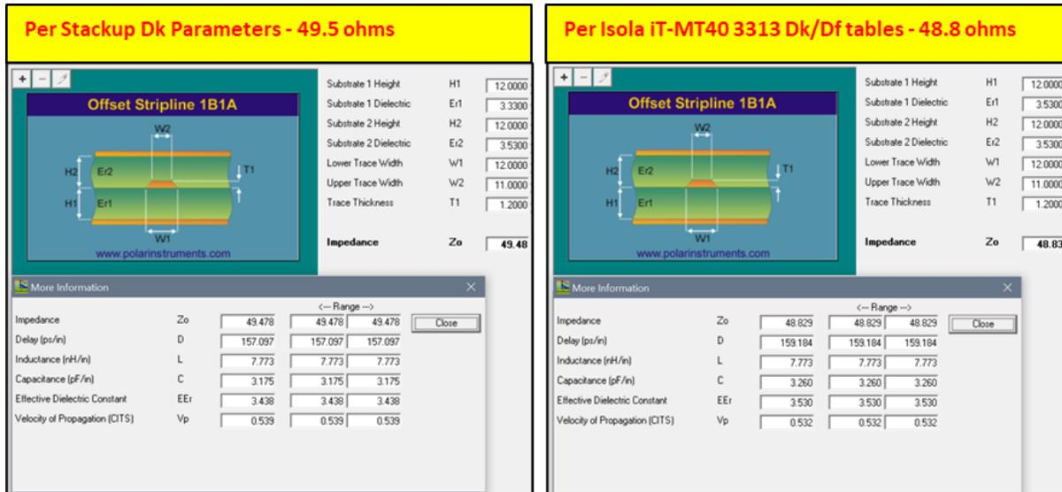
Figure 7 Comparison of characteristic impedance for 50-ohm trace using Dk for 1067/2x3313 core from stackup drawing vs Dk for 3x3313 from Dk/Df tables
