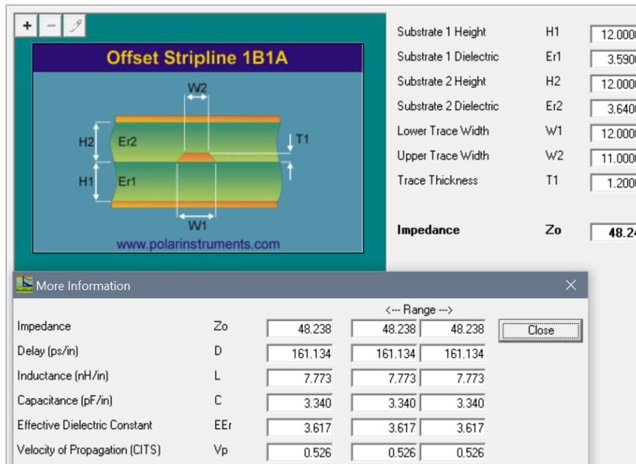
Figure 10 Polar Si9000 impedance prediction with Dkeff due to roughness
