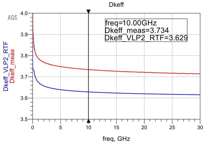
Figure 13 HLD Dkeff simulation correlation for as designed stackup
