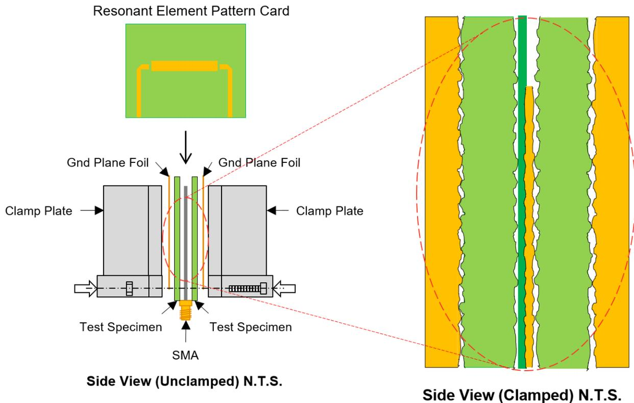
**Figure 3 Illustration of clamped stripline resonator test method, as described by IPC-TM-650, 2.5.5.5, Rev C, Test Methods Manual.**
