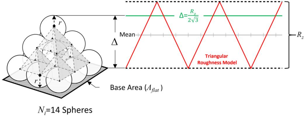
**Figure 4 Cannonball-Huray physical model. The height of the stack is the RMS height of the peak to valley profile equal to  $R_z$  from data sheets**
