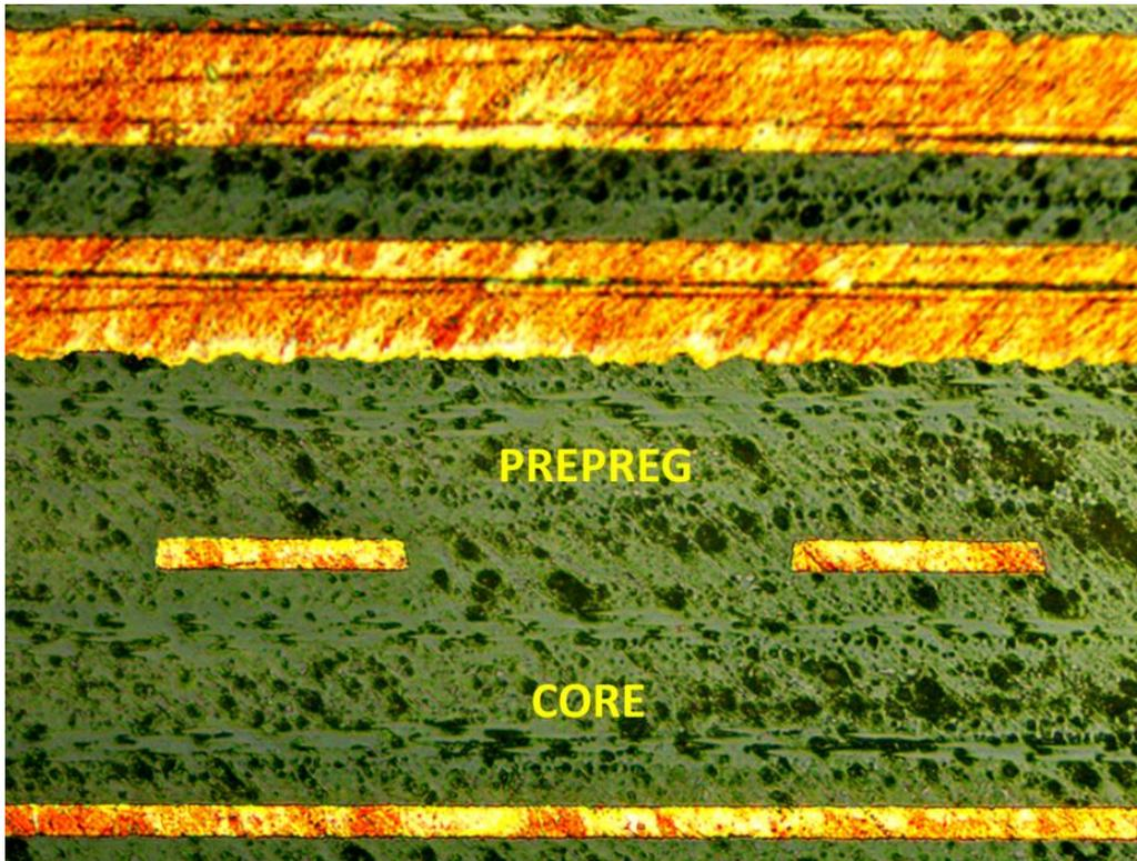
**Figure 1** An example cross-section stripline geometry from a stackup showing thin core laminate (top) with RTF bonded to prepreg and adjacent to a high-speed differential pair with smooth foil.
