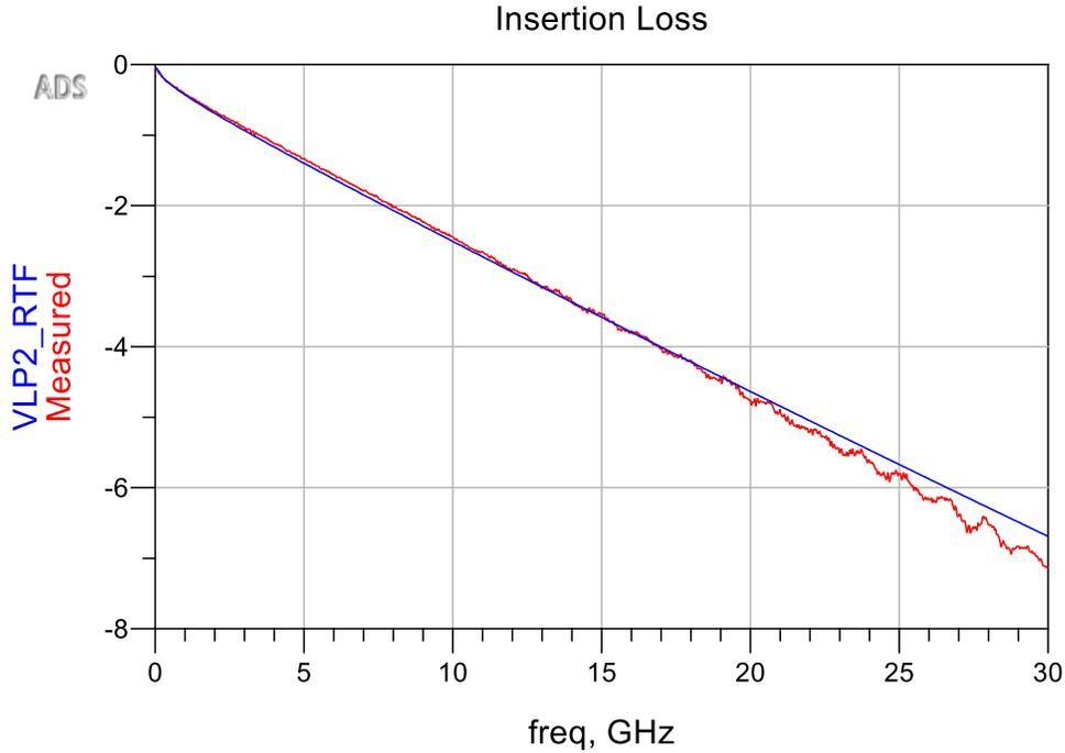
**Figure 12 HLD Insertion Loss simulation correlation for as designed stackup from data sheet and stackup parameters**
