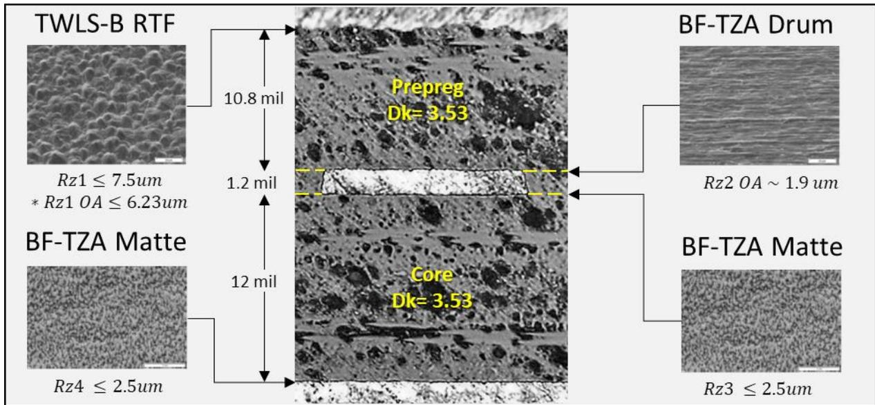
**Figure 9** Data sheet parameters for RTF/VLP2 foil roughness and dielectric properties for I-Tera® MT40 stackup geometry. Note: Photos are for illustrative purposes only and are not actual cross-sections from CMP PCB. Surface roughness pictures source: Circuit Foil [7]
