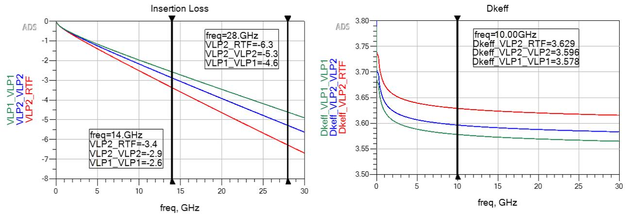
**Figure 15** What-if simulation comparison of VLP2/RTF, VLP2/VLP2, VLP1/VLP1 foil options and their effect on insertion loss and Dkeff
