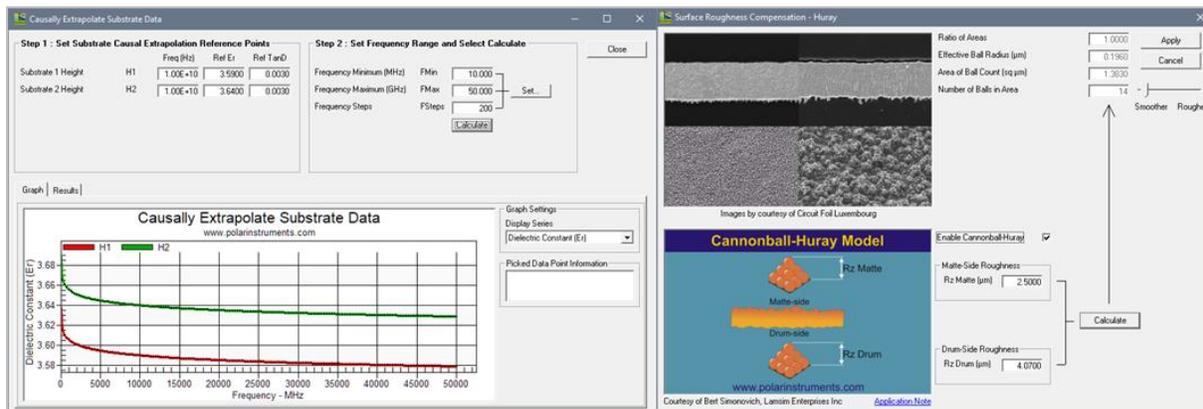
Figure 11 Causal Dkeff/Df dielectric and Cannonball-Huray roughness model input panels in Polar Si9000
