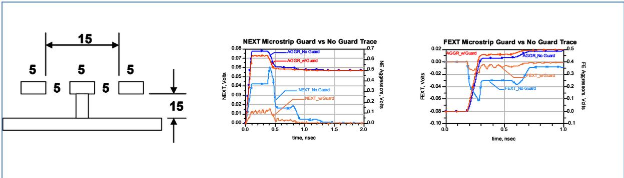
Figure 19 Scenario 2 Dielectric height increased to 15 mils, keeping all other parameters the same. The spikes and step in the NEXT and FEXT signatures are due to the impedance mismatch as seen by the Aggressor waveforms. Simulated with Agilent ADS.
