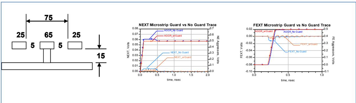
Figure 22 Scenario 5 Space increased to 3 times line width and guard trace increased to 65 mils to maintain 5 mil gap each side. NEXT and FEXT is comparable to the baseline case in Figure 18. Simulated with Agilent ADS.
