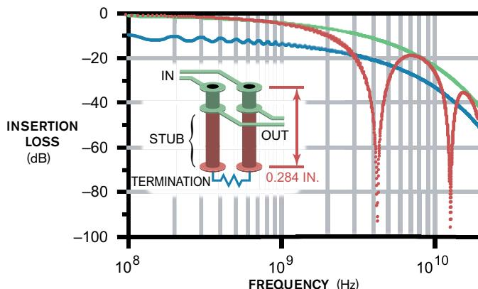
**Figure 1** In this simulation, using Agilent's ADS, the channel insertion loss represents two differential vias with 30 in. of PCB etch. This loss deteriorates significantly when you use long via stubs (red), as opposed to short, back-drilled vias (green).
