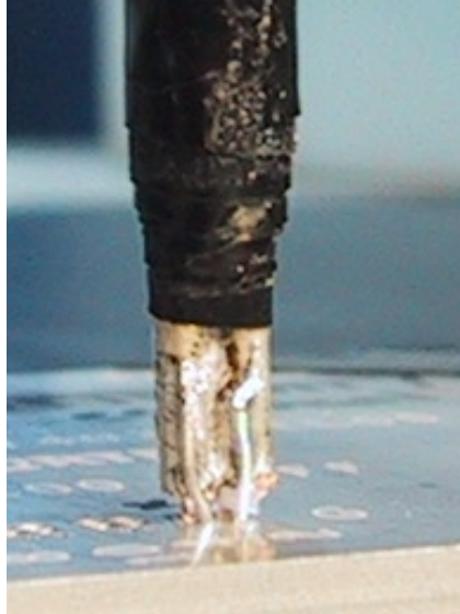
Figure 5. Close up of the custom, differential, semi-rigid coax probe tip.
